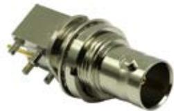
This right angle PCB connector is designed to give True 75 ohm performance offering exceptional low return loss up to 4.5GHz. This connector has a gold plated surface mount centre contact and has a fully machined main body. Supplied with a slotted circular fixing nut, Suitable tooling can be found in the Accessories and Tooling section of this catalogue.
