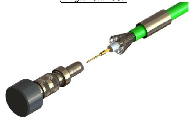
9. Slide the cable into the connector and push home until the centre contact "CLICKS" into place in the connectors dielectric. Ensure all the braid strands pass outside over the knurled area of the connector.
