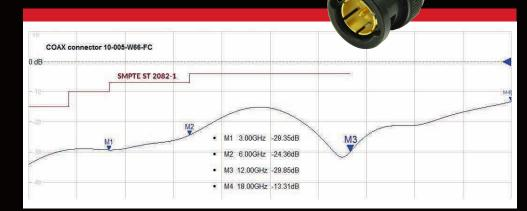
Now successfully tested to provide low loss performance up to 12GHz and in some cases 18GHz. The latest series of BNCs from COAX are perfect for new broadcast applications.
